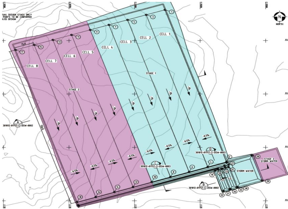
Figure 8: Castle Hill heap leaching pad design schematic
