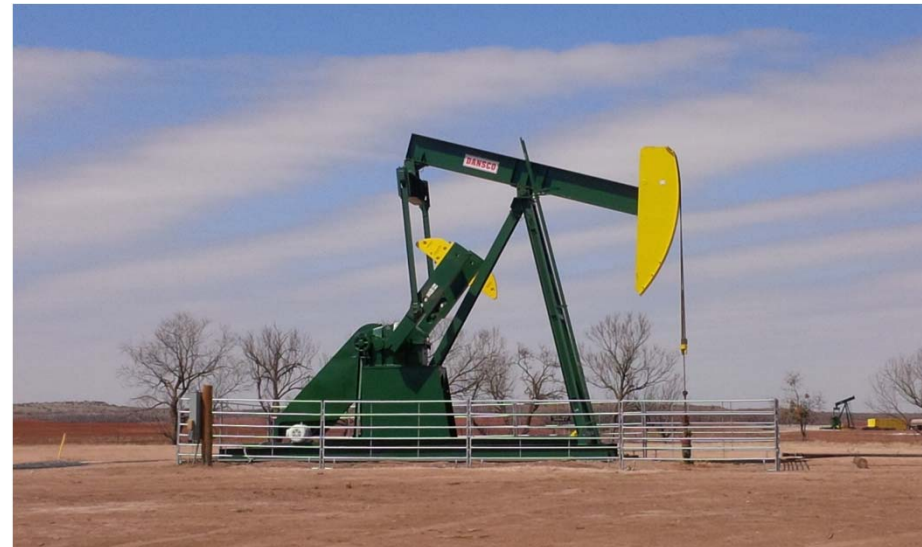
Typical Capitola vertical well lift system
