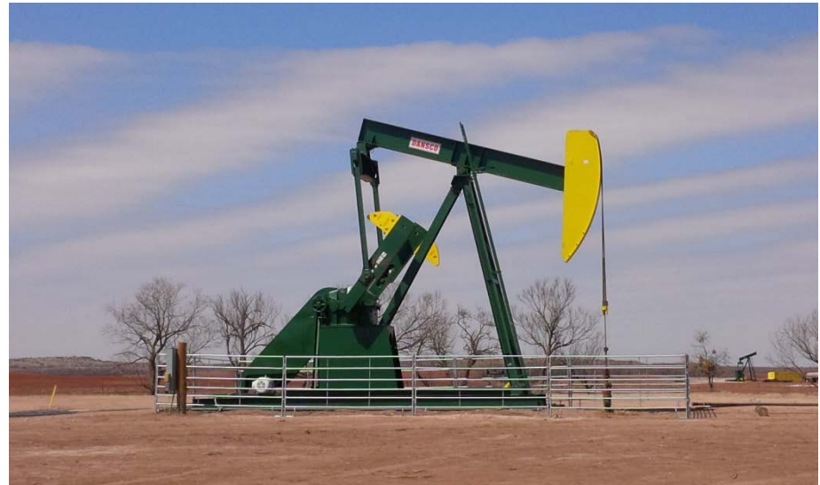
Typical Capitola vertical well lift system
