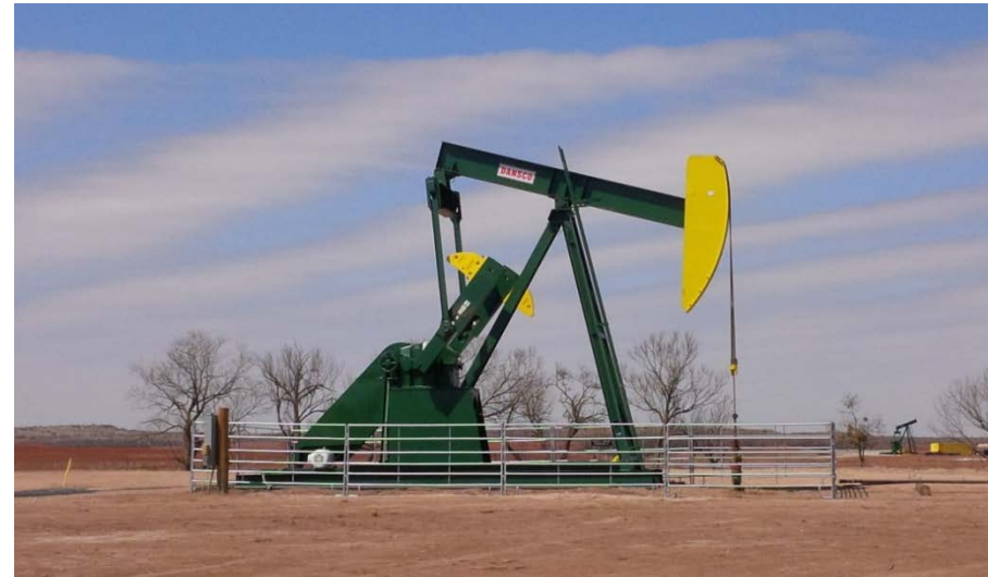
Typical Capitola vertical well lift system
