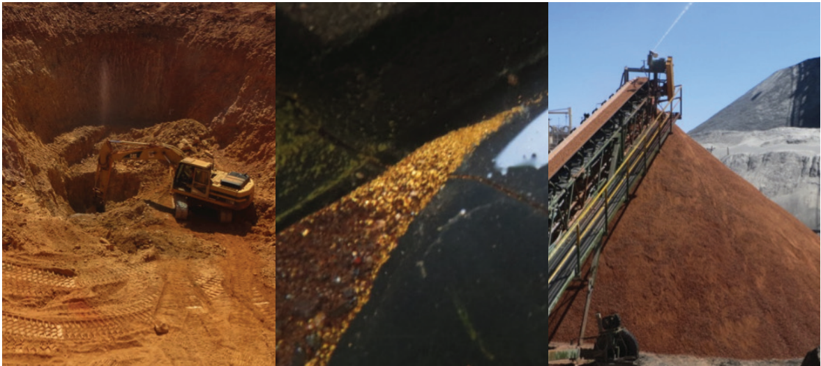
L-R: Base of Bulk Sample Pit - Excavating mineralised material for processing. Coarse gold panned from high-grade gold zone in 727 Bulk Sample Pit. Redcliffe Ore after crushing awaiting further processing.
