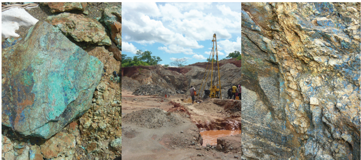
L-R: Malachite and azurite stains. Shallow diamond drilling on pit 2, Mbesa. Brittle to semi ductile shear with copper mineralization.
