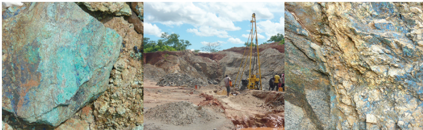
L-R: Malachite and azurite stains. Shallow diamond drilling on pit 2, Mbesa. Brittle to semi ductile shear with copper mineralization.
