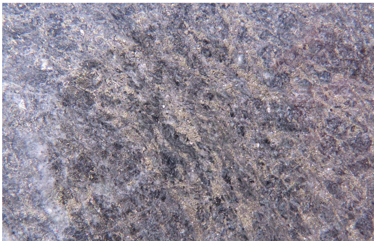
Figure 5: Matrix Sulphides ~270m in hole MFED042 (Field of view 8 x 4 cm). Grade is 2-3% Ni
