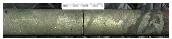
Figure 3: VUD 3, massive pyrite/chalcopyrite (NQ drill core)
