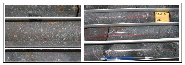
Figure 6: Left: VUD 7 drill core showing disseminated pyrite/chalcopyrite within a hematite matrix-rich breccia. Right: VUD 17, similar style of breccia and mineralization to VUD 7 at left (NQ drill core).
