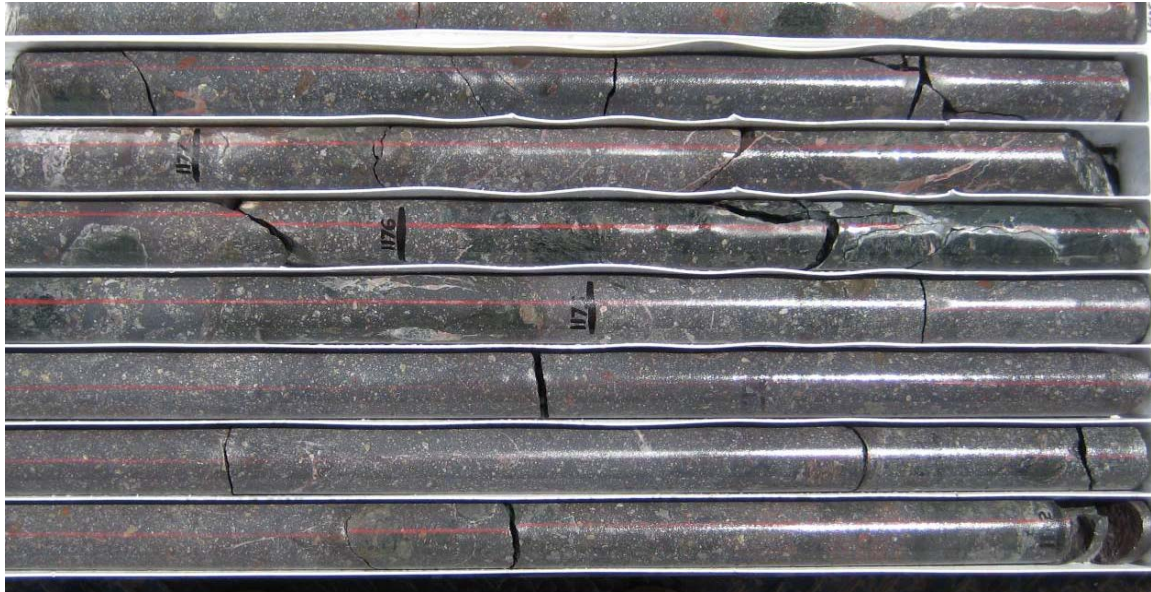
Figure 5: VUD 17: Mineralised hematite-rich breccias. The grey mineral is hematite (iron oxide) and the fine grained lighter coloured minerals are the sulphides pyrite (iron sulphide) and chalcopyrite (copper iron sulphide), and carbonate minerals (NQ drill core).
