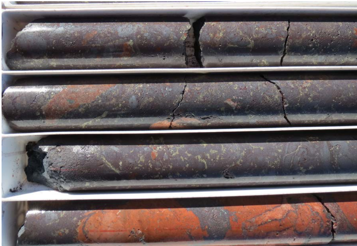
Figure 4: Detailed photo of mineralised hematite breccias within VUD 15. The grey/black mineral is hematite (iron oxide), the main, lighter (pale yellow) mineral is pyrite (iron sulphide) with chalcopyrite (copper-iron sulphide) and the red material at the base of the photo is a fragmented dyke.
