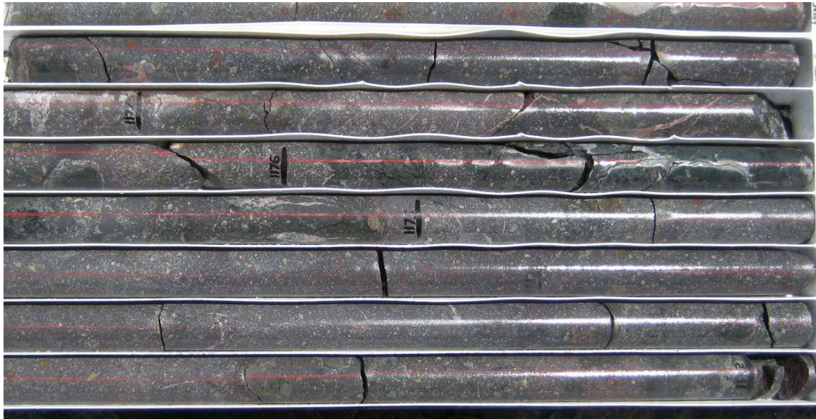
Figure 7: VUD 17: Mineralised hematite-rich breccias. The grey mineral is hematite (iron oxide) and the fine grained lighter coloured minerals are the sulphides pyrite (iron sulphide) and chalcopyrite (copper iron sulphide), and carbonate minerals (NQ drill core).
