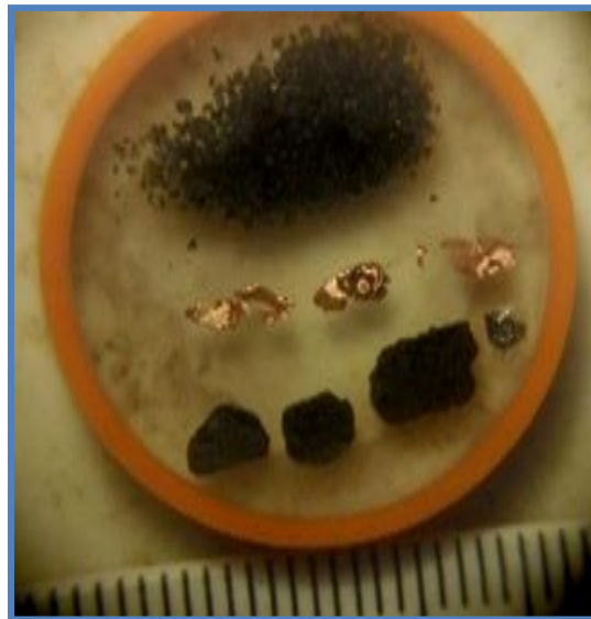
Figure 1. Native copper grains recovered from mafic drill chips from Hole TAZRC001
