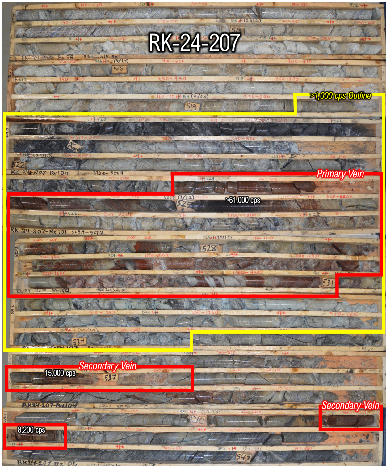
Figure 3: Core photo from RK-24-207; high grade mineralization is hosted across 7.1 m from 523.9 to 531 m with outer low grade disseminated uranium extending above to 519.4 and below to 534.4 m; Narrow secondary veins are hosted nearby in the footwall below
