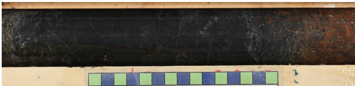
Figure 4: RK-24-207 close-up of off-scale (>61,000 cps) massive replacement by uraninite at 525.1 m
