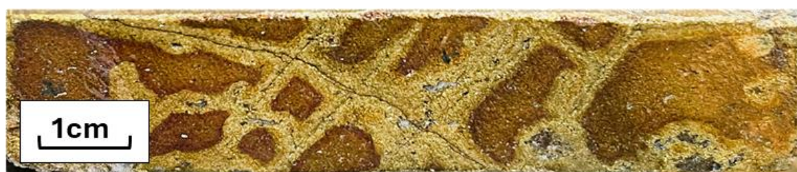
Figure 1: Photo of diamond core completed by Australian Oil & Gas Minerals Pty Ltd (1970's). Sample interval of 4.6 metres at 18.54 % Cu from 57.9 metres in TDH01 1 containing massive chalcopyrite (copper sulphide). Core diameter is BQ (36.4mm) with quarter core retained as a representative sample. Chalcopyrite is tarnished brown by length of time in core tray.
