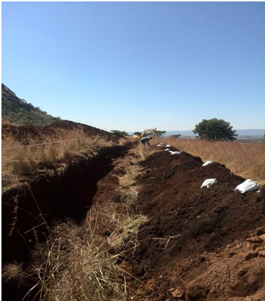
Fig 2: Trench sampling at Longonjo Rare Earth Prospect
