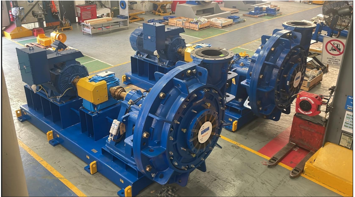
Figure 10: Cyclone Feed Pumps Ready for Collection (30 June 2025)
