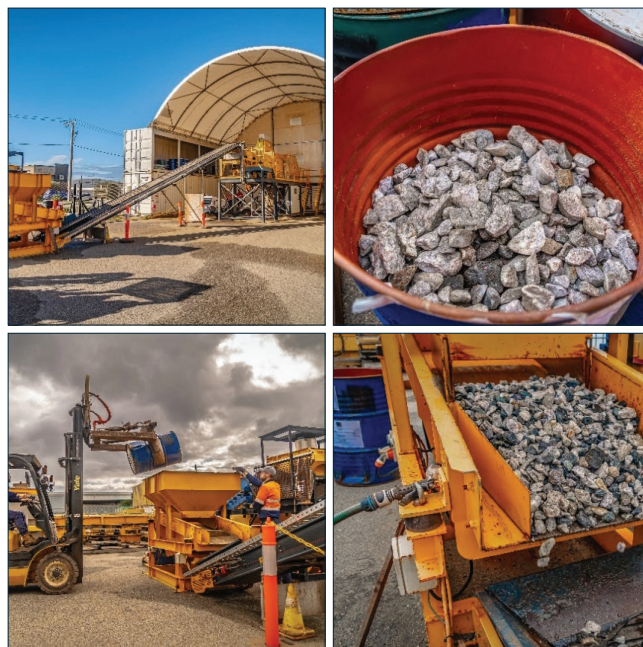
Figure 22 Shows the high-grade ore being processed through the Steinert ore sorting facility.
