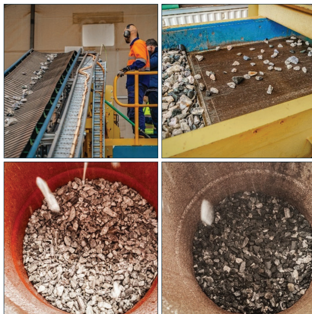
Figure 23 Showing Manna ore being processed through Steinert ore sorting facility.
