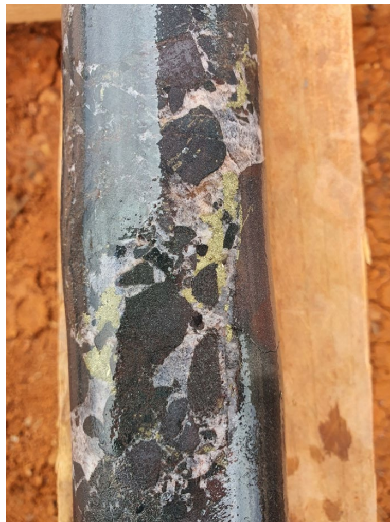
Figure 9 (left): Blebby/disseminated chalcopyrite in strongly haematized core, approx. 948m.
