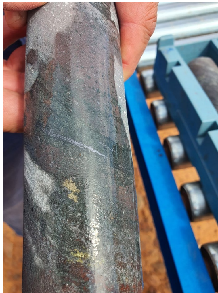
Figure 7 (left): Fracture filling molybdenite, approx. 929.5m.
