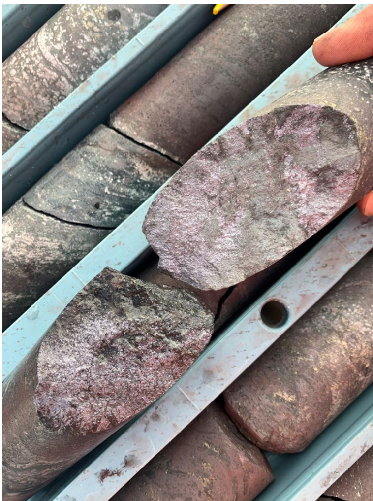
Figure 7 (left): Fracture filling molybdenite, approx. 929.5m.
