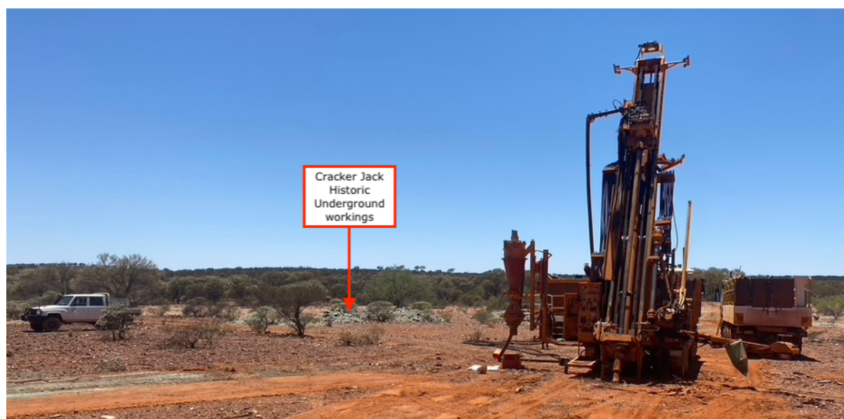
Photograph 1: Reverse Circulation (RC) drill rig at Cracker Jack prospect, part of the 100% owned Reedy South Gold Project.
