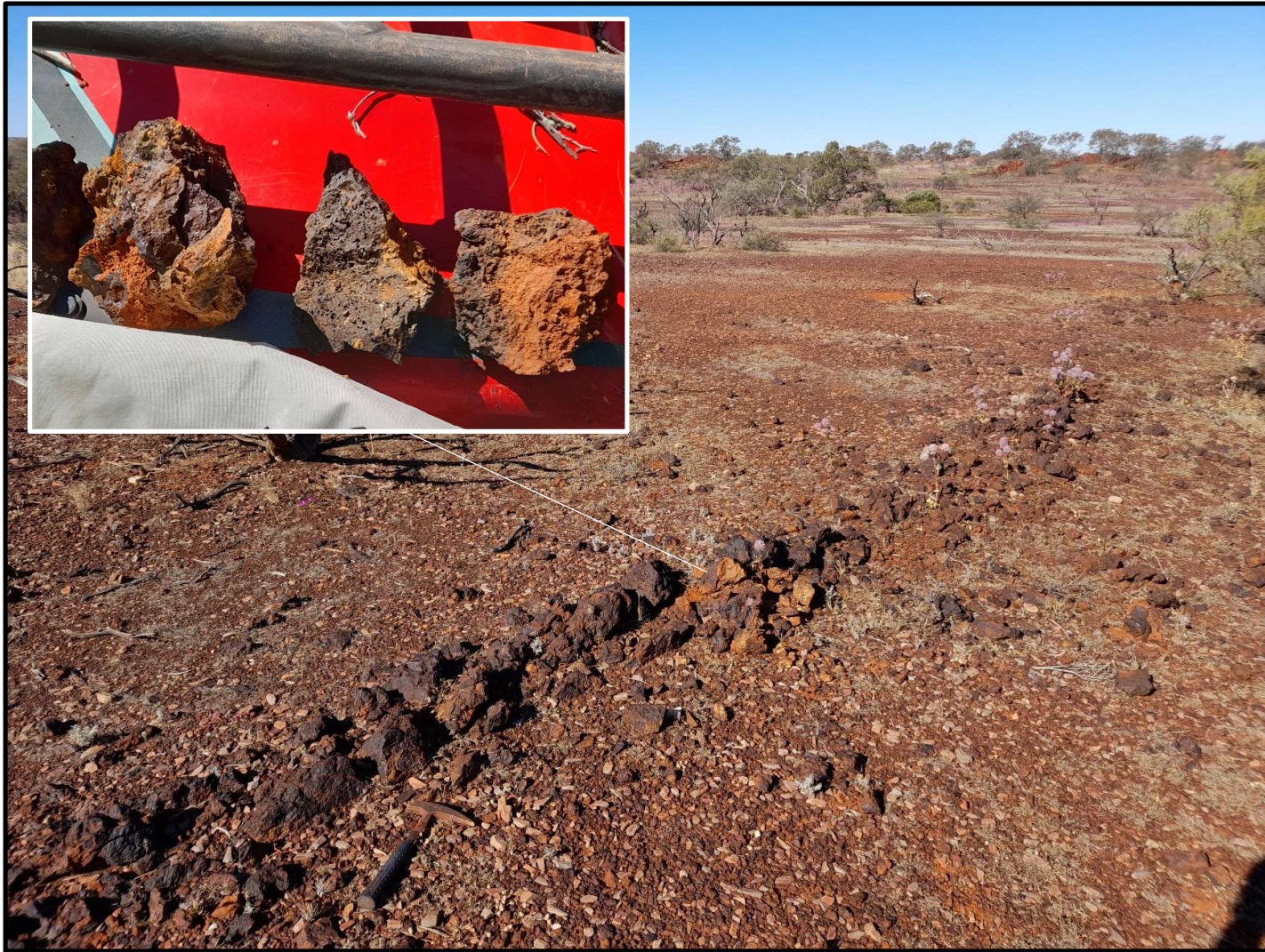
Figure 4. Gossan outcrop from EL 09/2422 with gossan specimens below showing boxwork after sulphide (Location: c. 368,400E 7,374,500N GDA94 Z50).
