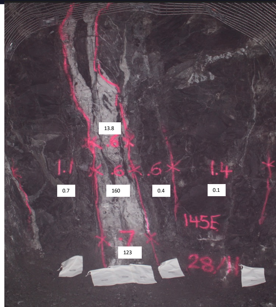
145E OD1 Face 112 (SOE Lode) – Currently Stopping Local Grid: -2067N, -695E, -139mRL
