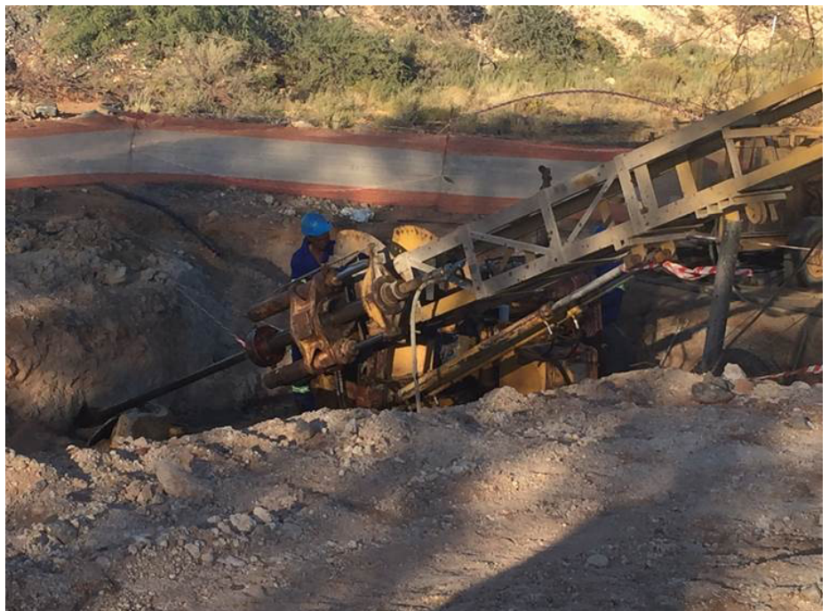
Figure 1: Shallow angle diamond drilling at the PC Project.
