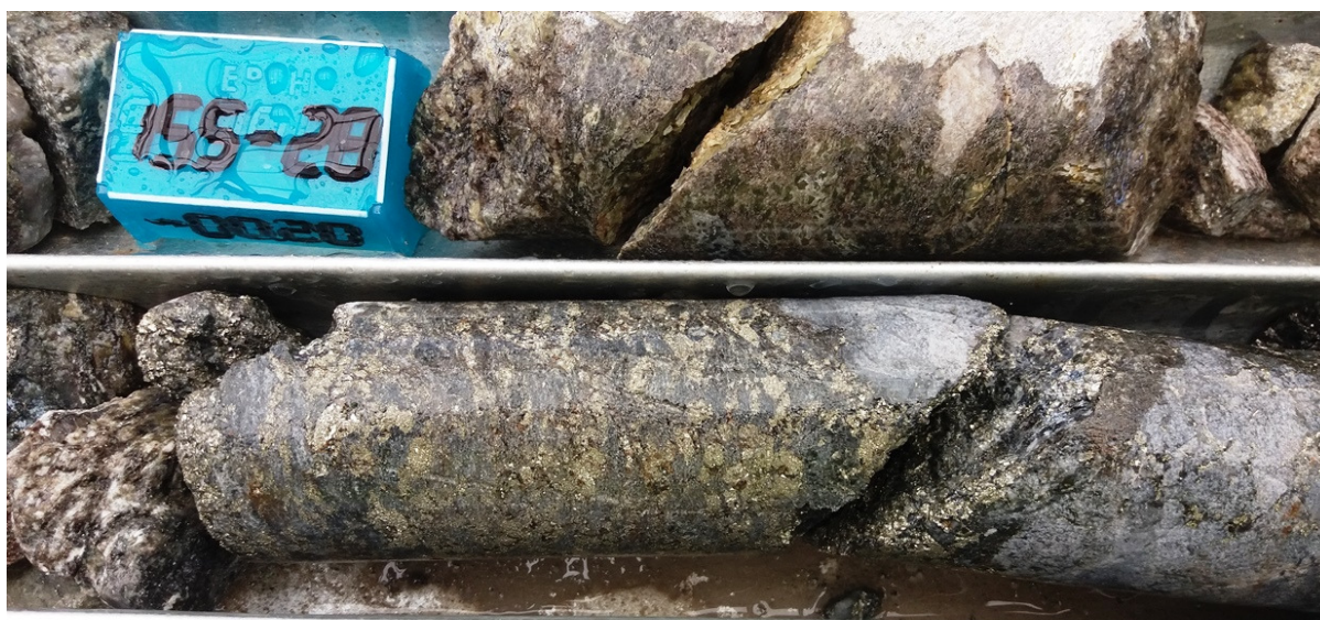
Figure 2: Massive sulphides in OCOD035 (157.8m downhole, approximately 80m below surface) at the PC Project.
