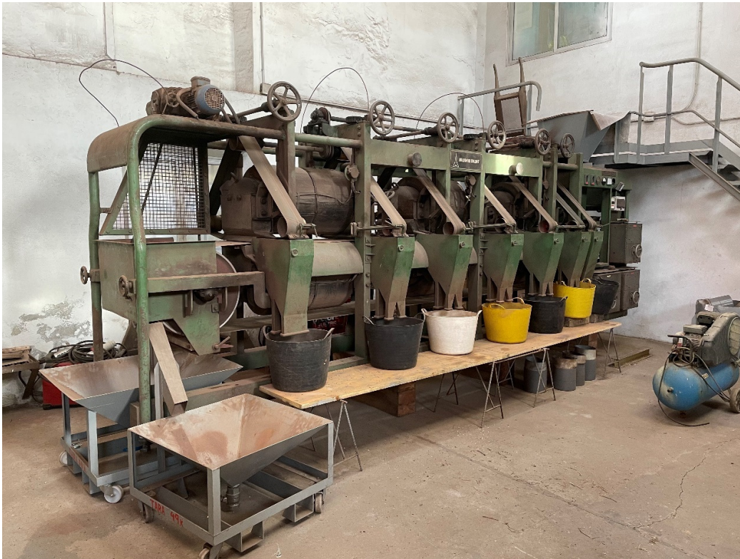
Magnetic separator used in the final stages of producing separate high-grade tin and tungsten concentrates
