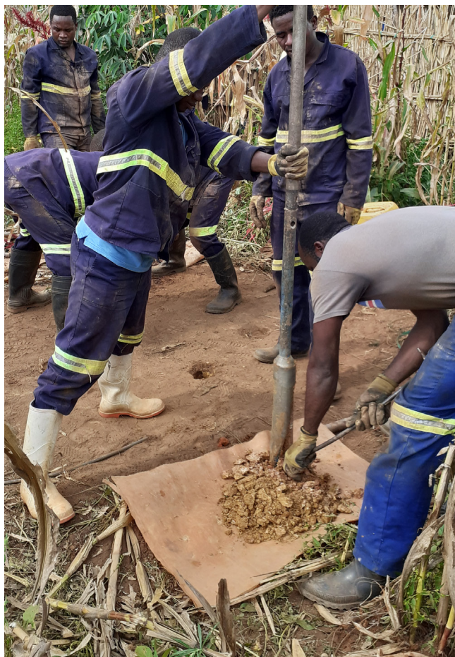
Figures 6-7. Sovereign team members hand-auger drilling at Kasiya.
