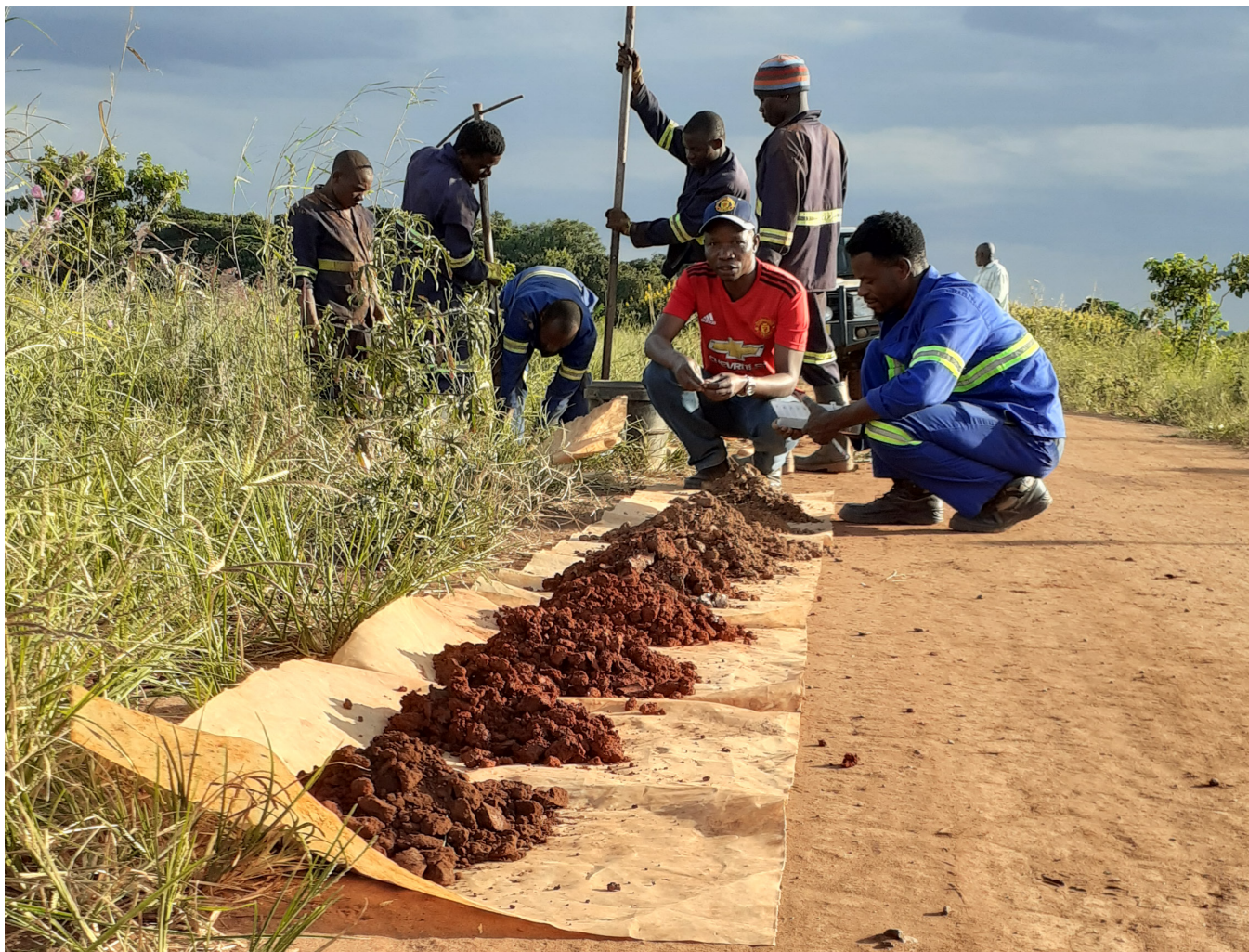
Figure 3. Logging of rutile hand-auger samples at Kasiya.
