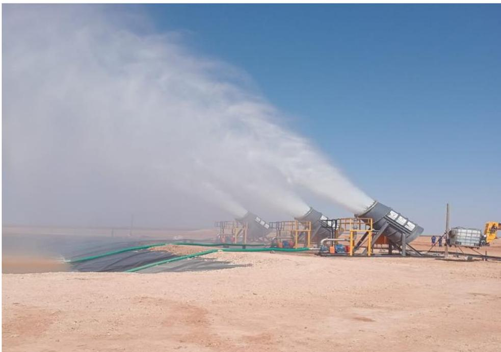
**Photo 1: Water evaporation on site at PCZM.**
