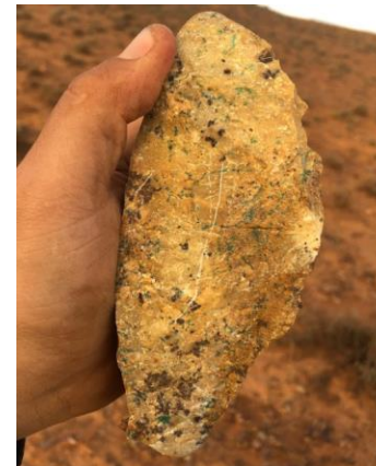
Photograph of malachite in sample WK0266, 2km north of sampling at Woolshed adjacent to the high magnetic anomaly which assayed at 1.7% Cu.
