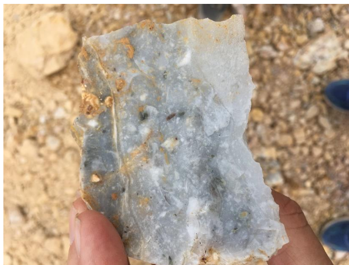
Figure 1. Chalcedonic quartz from Mongyu Mine, (excised from the Mongywang Application area). This type of quartz veining is characteristic of shallow level of low-sulphidation gold systems such as Vera Nancy in Queensland. Higher gold grades are usually found deeper down in the system, below the current shallow open pit mine.
