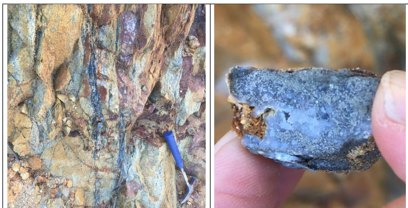
Figure 6. Sheeted quartz-pyrite veins within the Loi Kham Lone open pit (left) and a close up of quartz-pyrite vein material.
