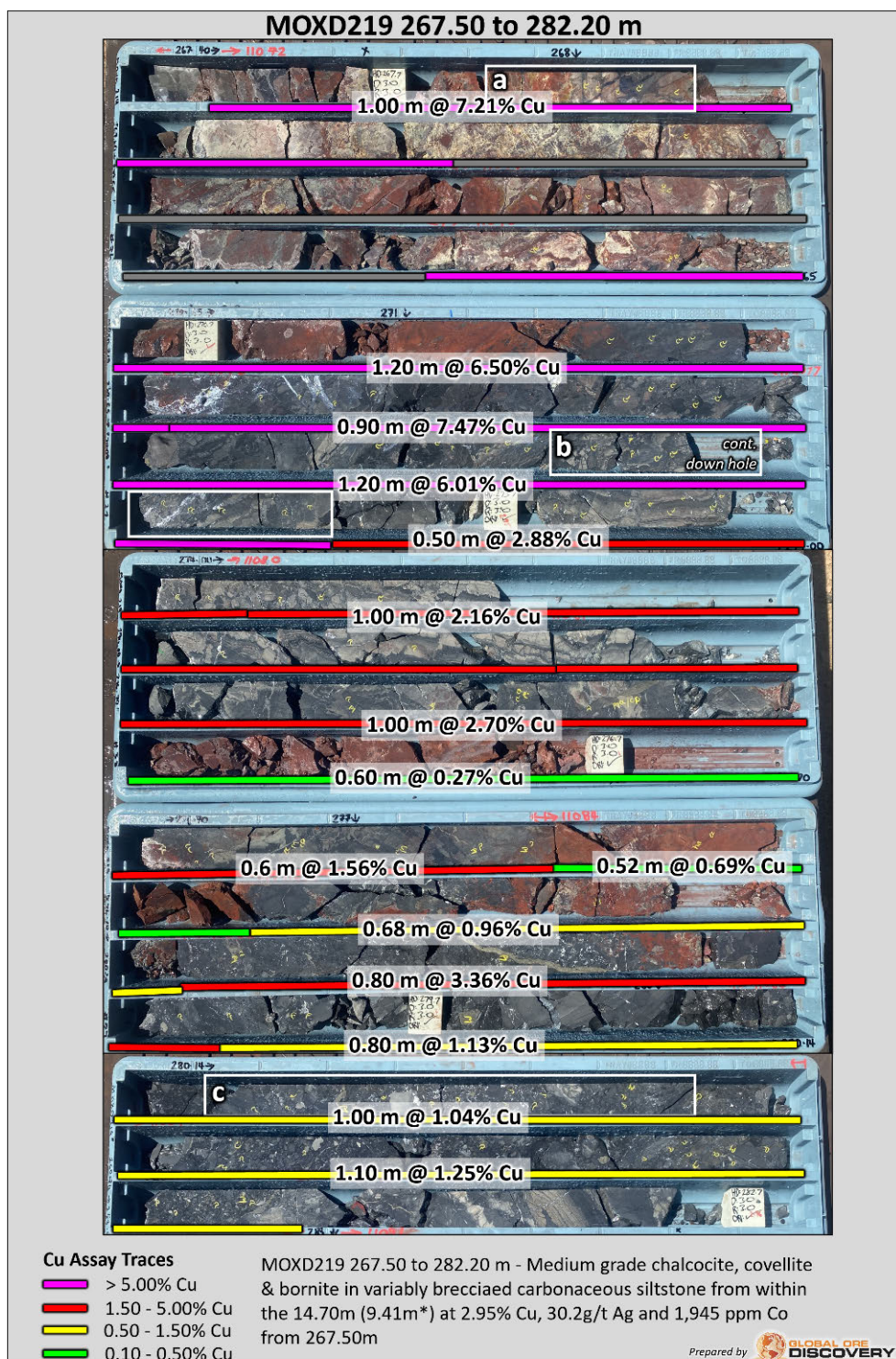
Figure 6. MOXD219 267.50 to 282.20m - Chalcocite, covellite & bornite in variably brecciated carbonaceous siltstone from within the 14.70m (9.41m*) at 2.95% Cu, 30.2g/t Ag and 1,945 ppm Co from 267.50m downhole.
