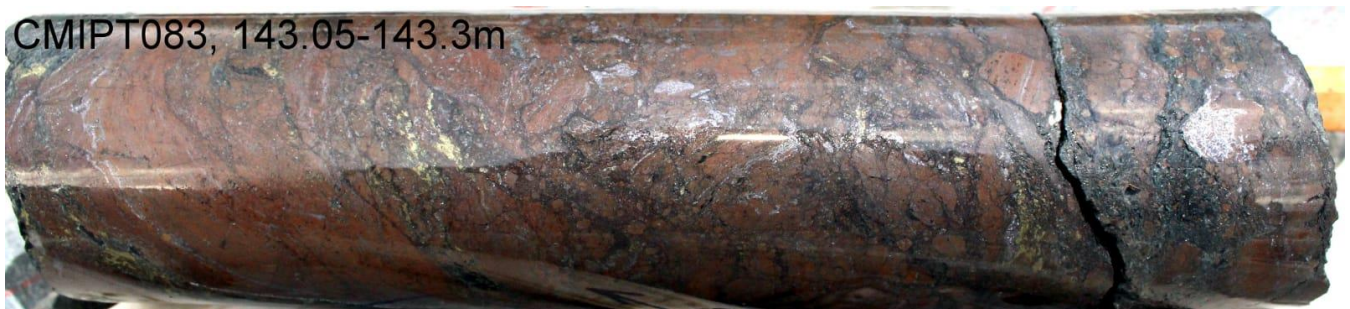
Figure 5. Hole CMIPT083: high-grade massive and brecciated massive sphalerite (red-brown) with lesser galena. Up to 3% chalcopyrite (yellow) is present in places.
