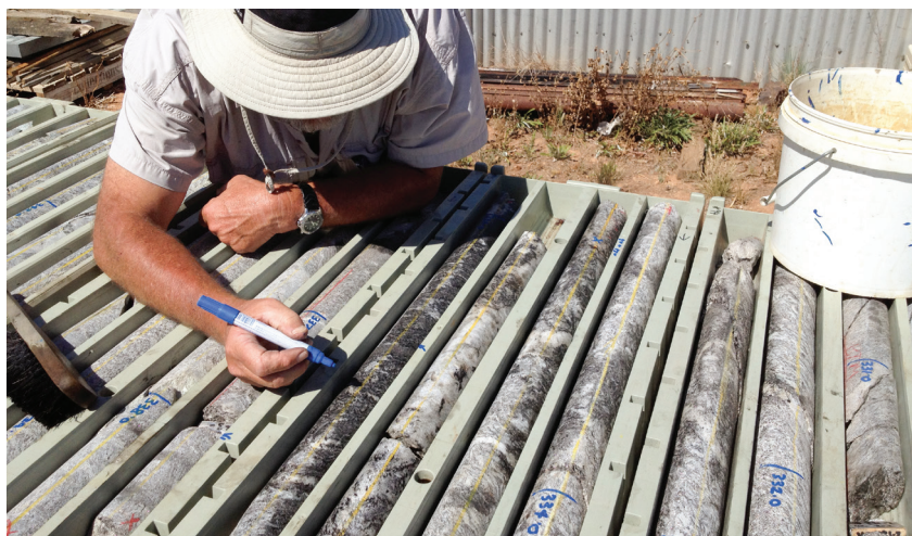
Thackaringa – Logging Diamond Drilling Cores
