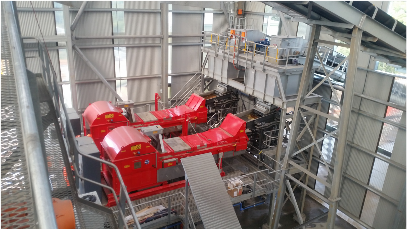
FIGURE 2 : RENISON ORE SORTER XRT MACHINES
