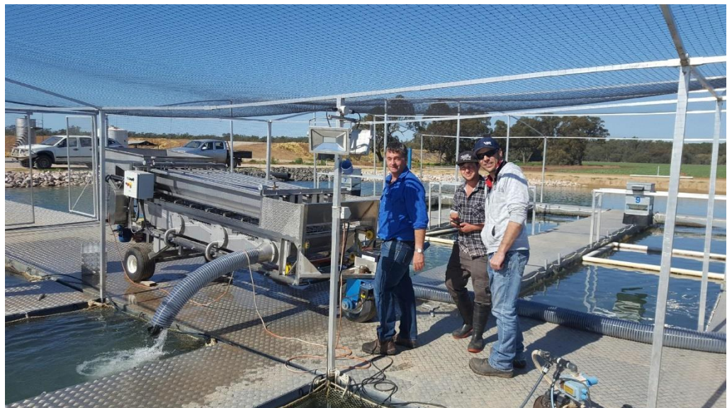
Picture 6: Fish grading machine operating on contractor grower farm
