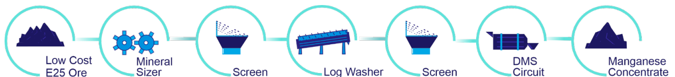
Figure 8: Butcherbird Schematic Flowsheet.
