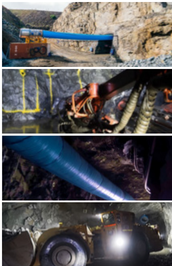
Photos from top: Decline portal access from Christmas Pit; Underground decline development; Jumbo boring face; Underground LHD bogger.
