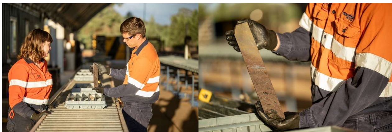
Figure 2: Nymagee District Exploration Geologists displaying drillcore from (left) hole FDD219W1, between 446.5m and 446.7m, showing massive sulphides consisting of banded red sphalerite (ZnS), silver galena (PbS) and bronze chalcopyrite (CuFeS 2 ), and (right) hole FDD219, between 489.6m to 490.0m, showing banded, massive yellow and red sphalerite (ZnS), silver galena (PbS) and black chlorite.
