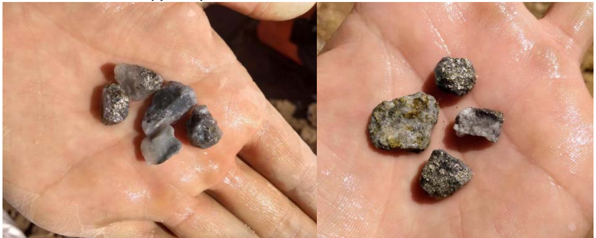
Photo 4 (left). Hole LORC19-03, Rock Oven Target vein. Crystalline and chalcedonic quartz, with some banded chalcedonic quartz: pyrite sphalerite, black silica. Photo 5 (right). Hole LORC19-03, Rock Oven Target vein. Massive sulfides: pyrite, arsenopyrite, sphalerite, jarosite, some chalcopyrite.
