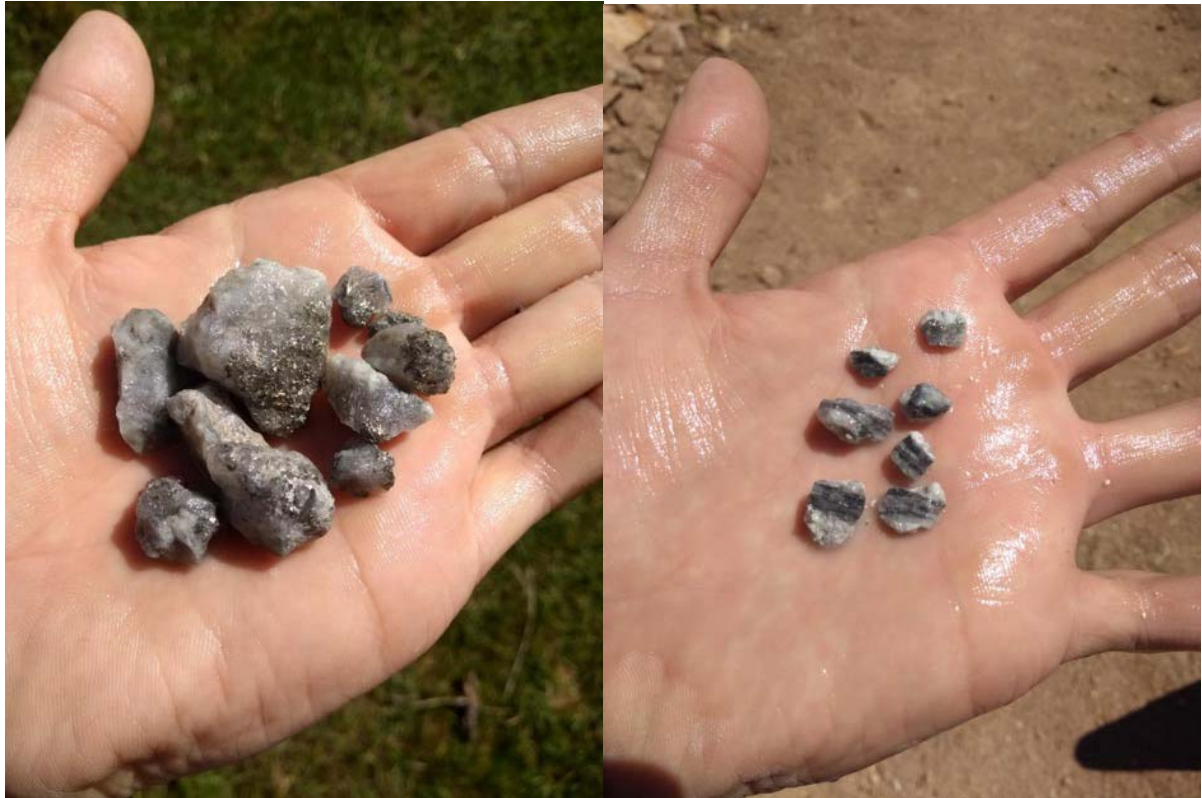
Photo 2 (left). Hole LORC19-01, Rock Oven Target vein. Crystalline quartz with pyrite, sphalerite and arsenopyrite, some argillic alteration. Photo 3 (right). Hole LORC19-02, Rock Oven Target vein. Sulfide banded veinlets: pyrite, sphalerite, black silica banded.
