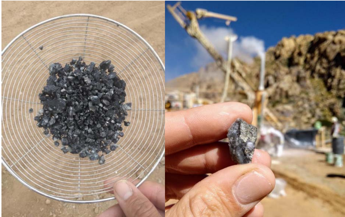
Photo 6 (left). LORC19-07, Tramway Target vein. Sulfides in chalcedonic quartz vein-breccia: pyrite, sphalerite, arsenopyrite. Photo 7 (right). LORC19-07, Tramway Target vein. Chalcedonic quartz vein with some brecciation: red sphalerite, pyrite, some chalcopryite.
