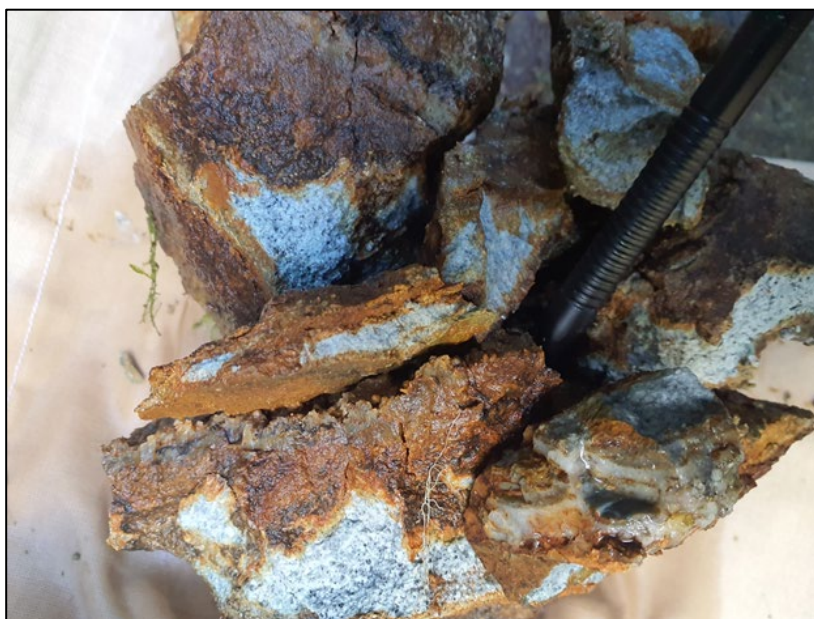
Figure 4. Example of Mineralization from the Lumuni Outcrop. Chalcedonic, locally banded and recrystallized comb quartz forming on the walls of open vugs, and abundant strongly oxidized sulphides in intensely altered medium-grained monzonite. Pen for scale.
