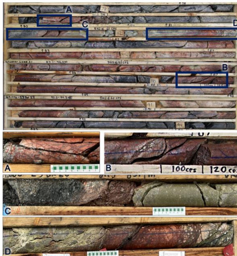
Figure 3: Photographs of alteration and deformation style intersected in a major faulted interval (shear zone) in drillhole GKI-006. A. Close-up of a hematized clast-supported crackle breccia with dark chlorite and hematite matrix. B. Close-up of strongly hematized fractured host rock with elevated CT-007-M scintillometer radiometry. Note the 3 cm-thick matrix-supported breccia exhibiting corroded clasts within a friable fine grained hematitic clay matrix. C. Close-up of a strongly altered cataclastic interval consisting of an incohesive gouge with dark grey to light grey clay matrix (left), an incohesive brick-red protobreccia (middle), and an indurated ultracataclasite zone with a sage green chloritic matrix (right). D. Close-up of continued strongly altered brecciated interval with brick red hematite noted overprinting the middle section of the photographed core and a later reactivation stage marked by a pale green-yellow clay matrix supporting chlorite-altered clasts.
