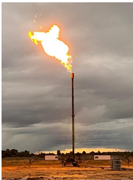
Gas flare of approximately 3 MMSCFPD from Daydream-2
