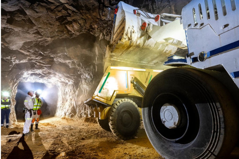
Photo 1: Trial Mining at PCZM. Geotechnical conditions in this 50-year-old excavation allow large stable excavations for mechanised mining.
