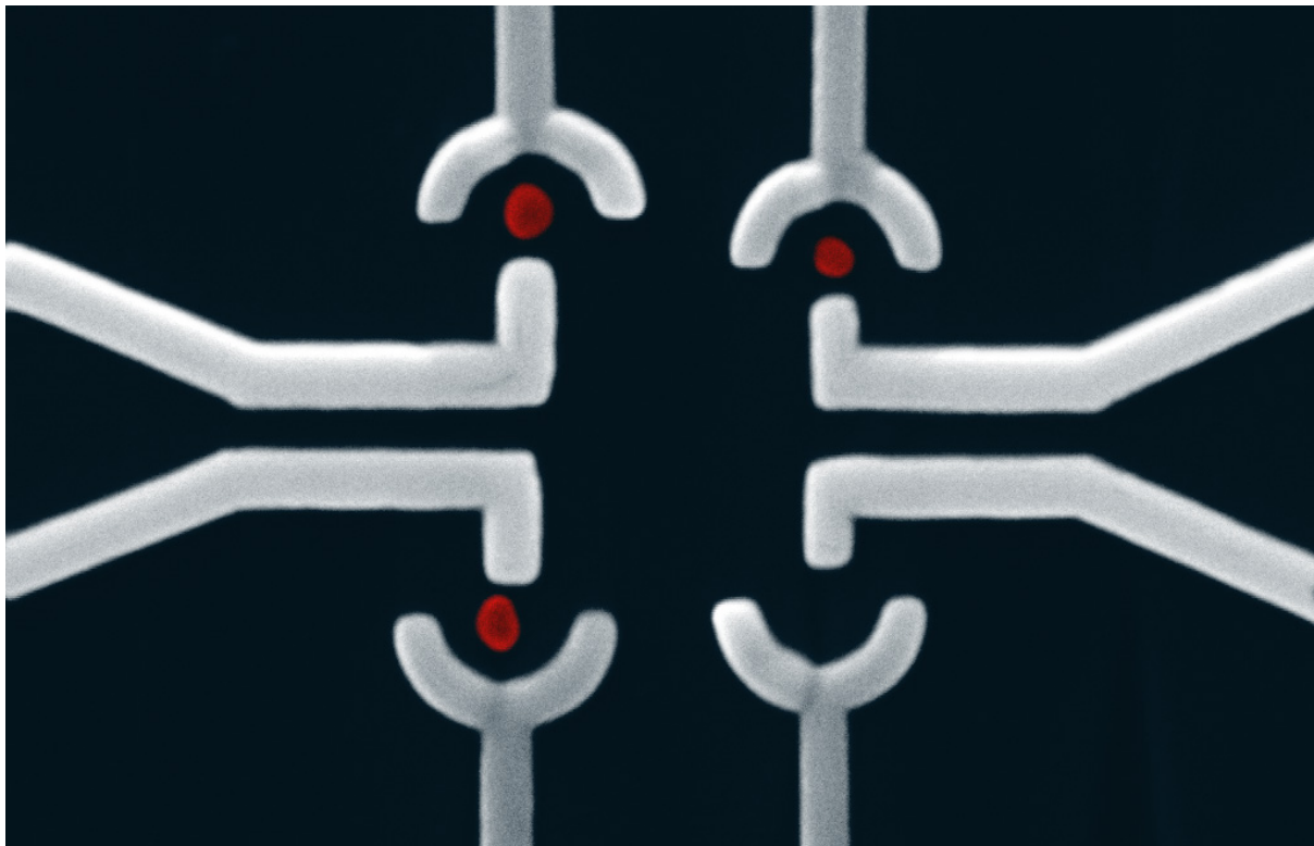
Fig. 1. Electron microscopy image of three isolated qubits (spherical shapes false-coloured in red-orange), positioned into an array on a silicon wafer surface, with each approximately 50 nanometres in size. Metallic control electrodes (false-coloured in grey-blue) aligned with nanoscale precision to the qubits. The width and height of the electrodes are comparable to the dimensions of the qubits, and compatible with modern electronic device features.
