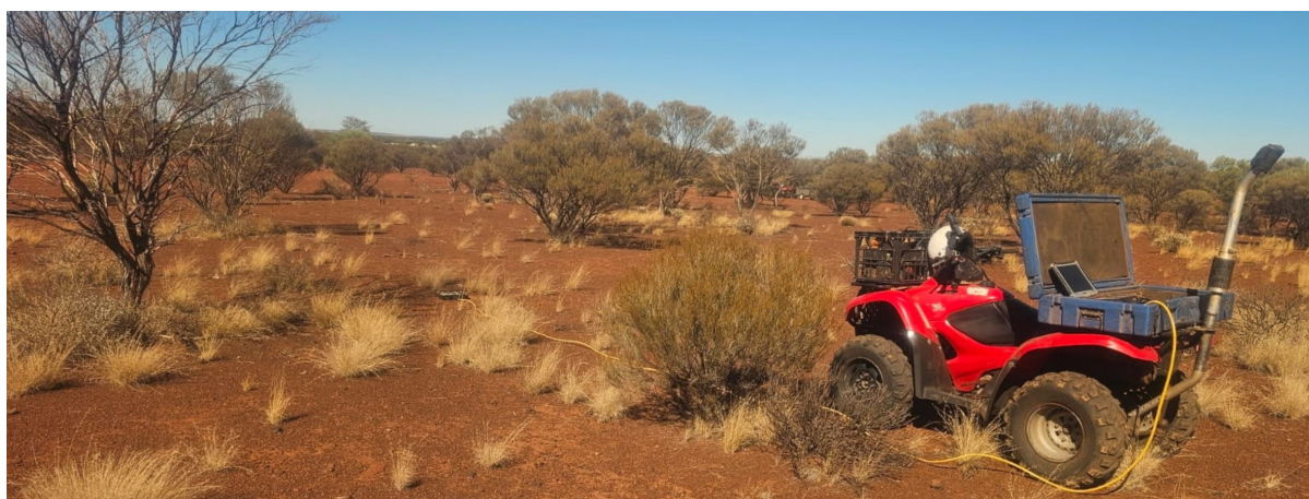
Figure 2: MLEM survey underway at the Ilgarari Copper Project.
