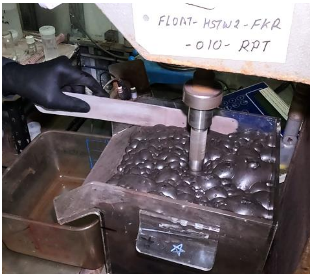
Figure 3. Bench scale saline water flotation testwork at Bureau Veritas laboratories, Adelaide
