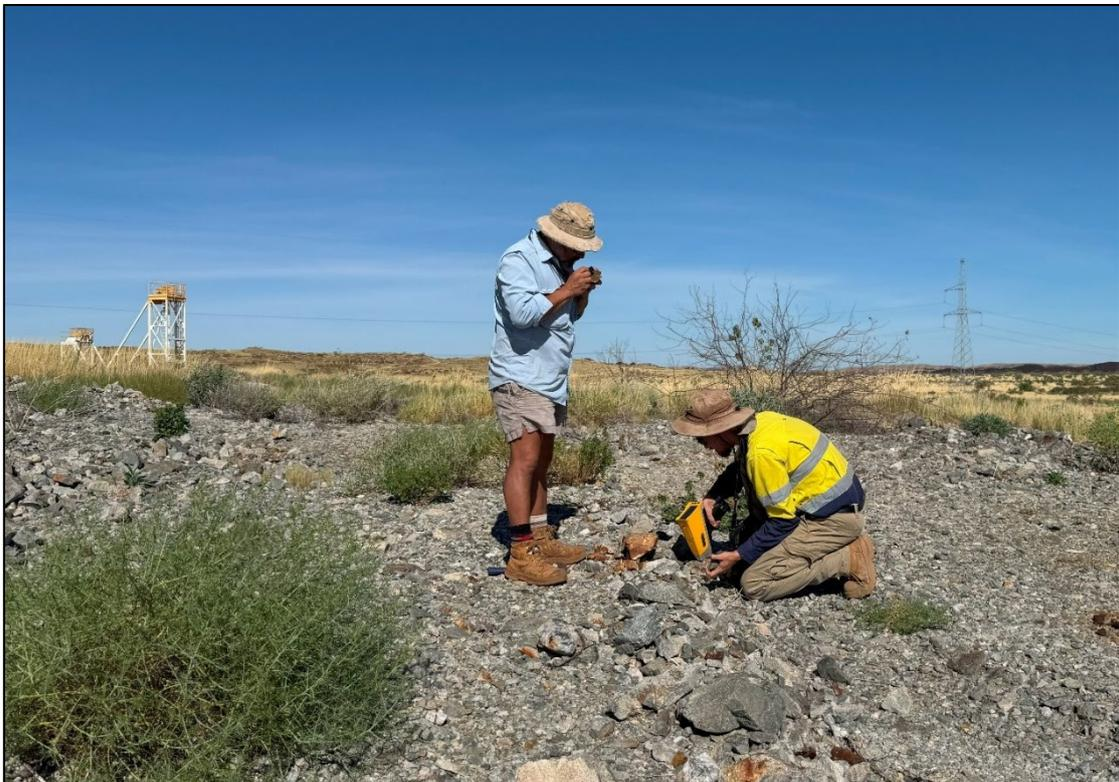
Figure 1 – Errawarra’s geologists on site at Elizabeth Hill. Geologists in the foreground analysing utilising pXRF technology and Elizabeth Hill headframes in the background.
