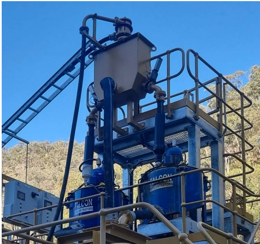
Figure 10 Reward gravity gold Falcon concentrators
