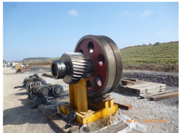
Drag/hoist input pinions
