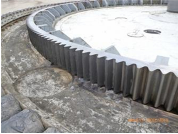
Tub cleaned and swing rack re-lubed
