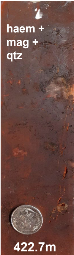
Zone of strong hematite IOCG style alteration (rust red colouration) in hole ABNE 2 (interval 417.9m – 426 m)
