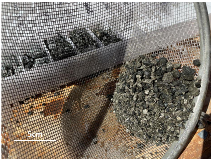
Massive sulphides in RC drill chips (207m, MIRC013)
