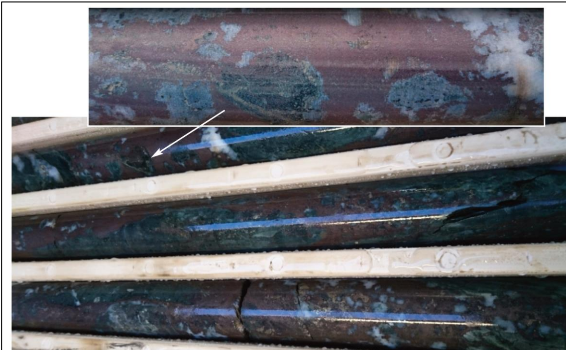
Figure 8: Photograph DDH cores showing Zn sulphide (sphalerite stringers) in DDH CWDD0001 from 486m depth. NQ2 (46.7mm diameter) DDH core within the tray with each length approximately 1m long.
