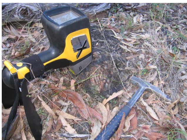
Subcrop of mineralised zone, showing moderate south dipping veins. Portable XRF unit was used in initial reconnaissance work, all results reported in this release are from chemical assays completed at ALS Brisbane
