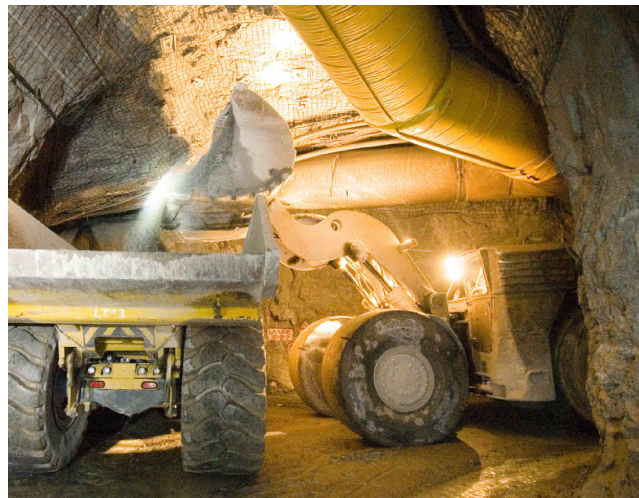
ABOVE: Underground during test mining loading rock into truck for haulage to the surface. This was at the 'Imperial mine, located about 5 kilometres from 'Central'. Future mining will be at 'Central' where there are many more reefs.
